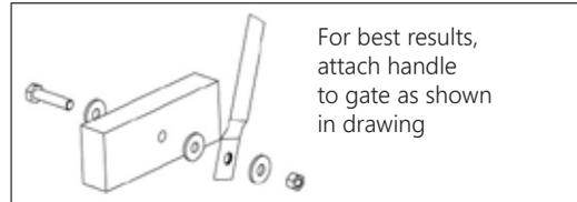
1. Decide where to fit the EASY LATCH®. Fitting between the 2nd and 3rd rails allows the handle to sit higher, which is preferred by horse riders.
