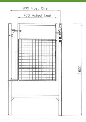
Gate height out of ground is normally 1.0m - 1.1m
